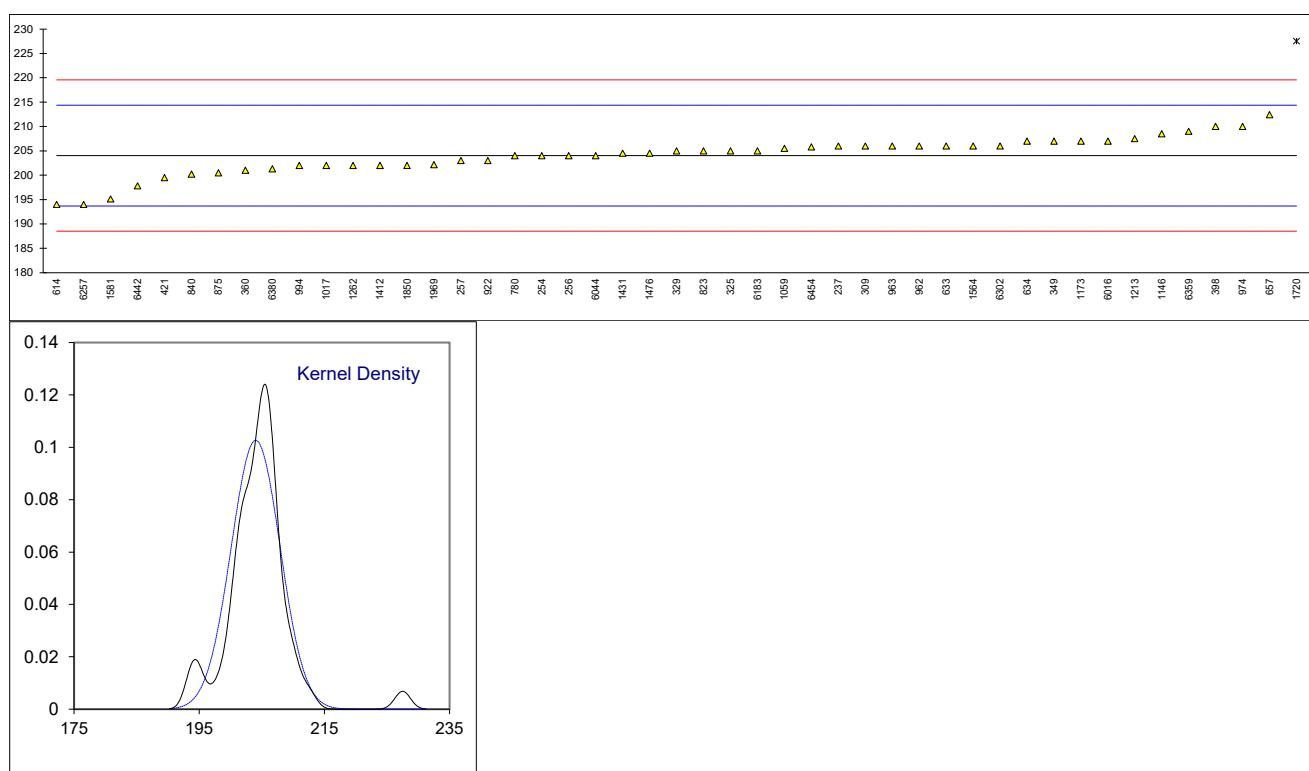
Determination of Kinematic Viscosity at 40 °C on sample #22085; results in mm<sup>2</sup>/s
