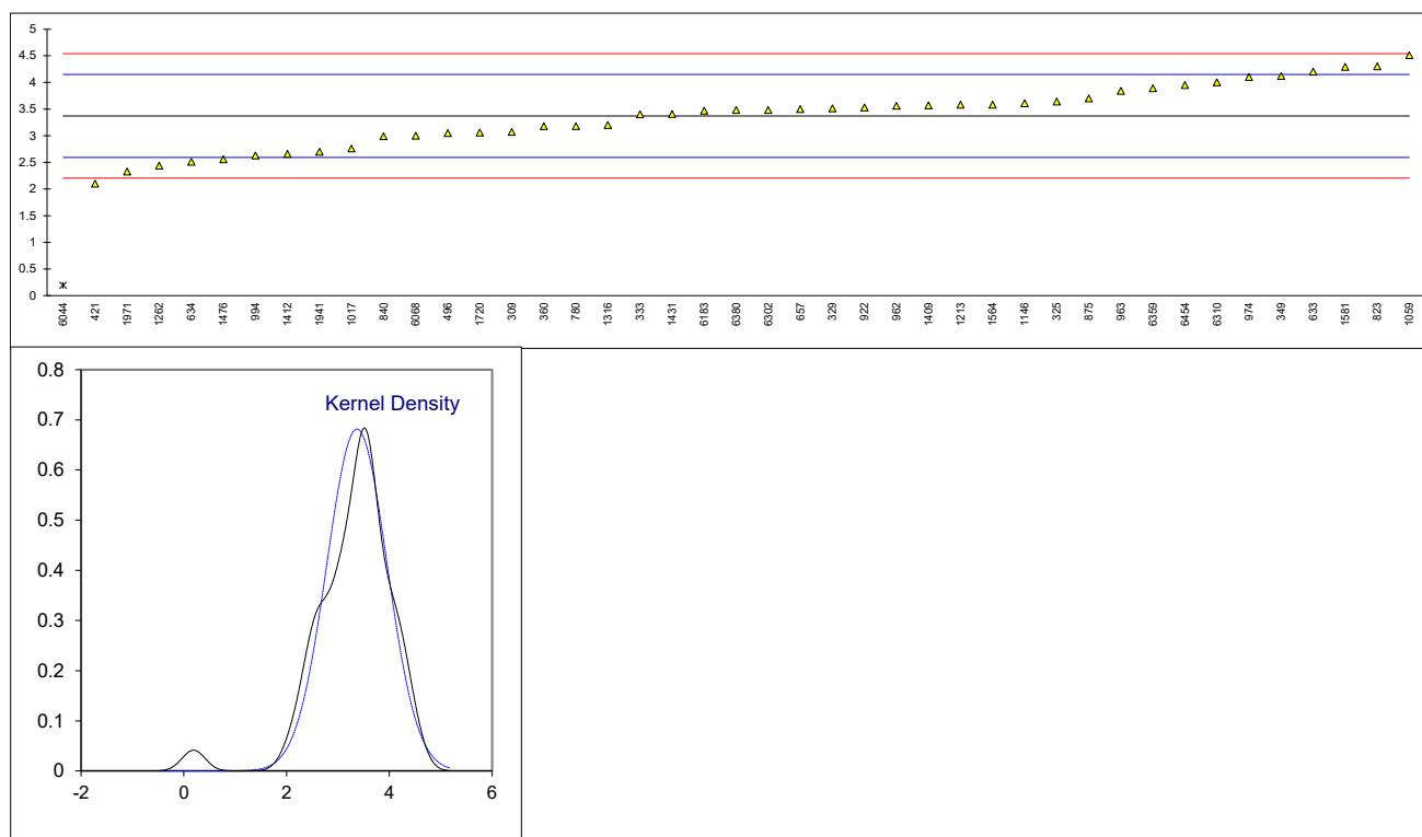
Determination of Base Number (HClO<sub>4</sub> titration) on sample #22085; results in mg KOH/g
