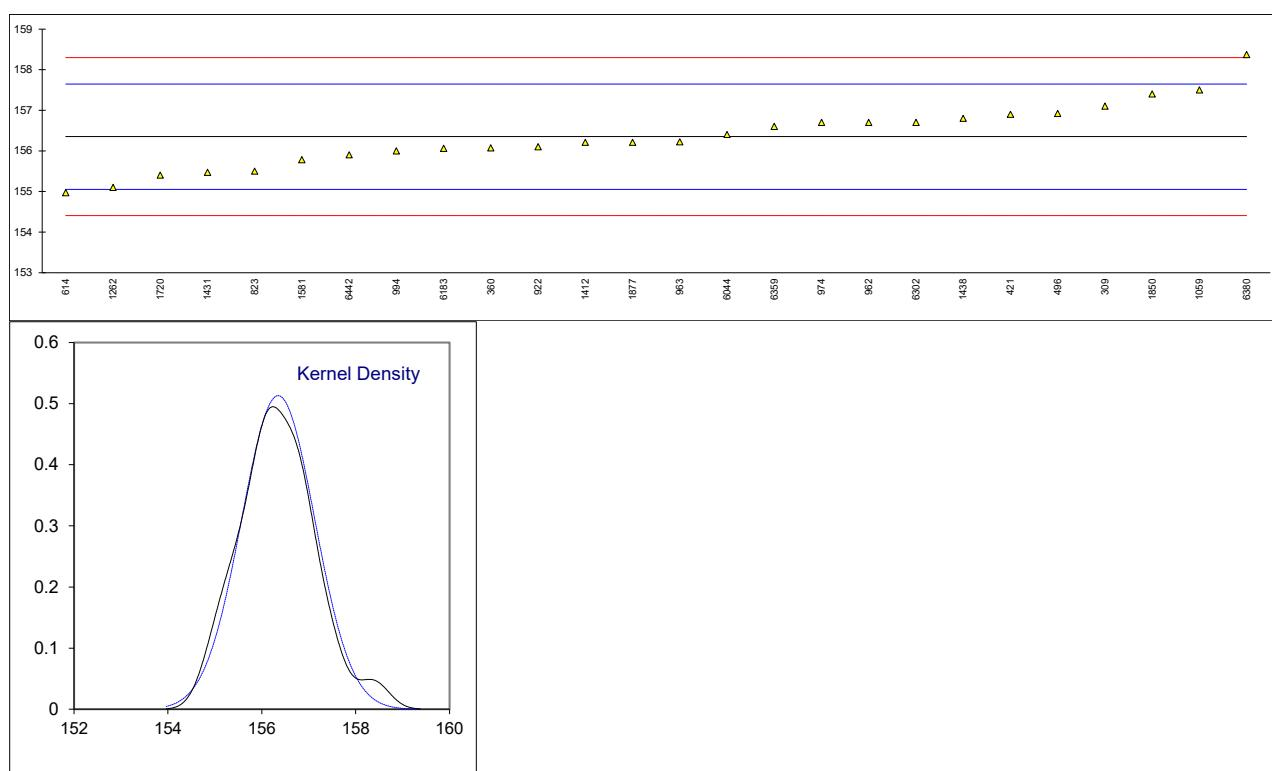
Determination of Kinematic Viscosity Stabinger at 100 °C on sample #22085; results in mm<sup>2</sup>/s
