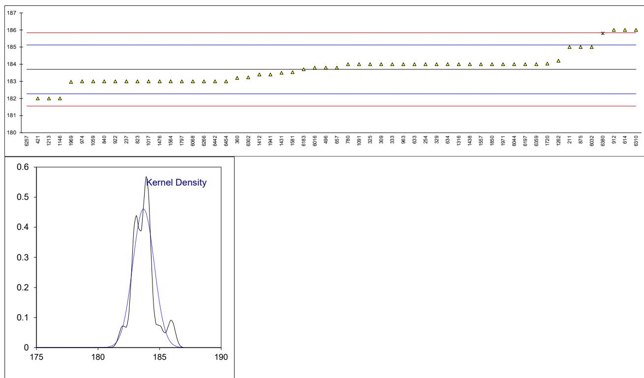
Determination of Kinematic Viscosity Stabinger at 40 °C on sample #22085; results in mm<sup>2</sup>/s
